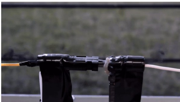
MC4 connector overheating \ melting which typically leads to hazardous DC arcs, courtesy of SolarDefend company
