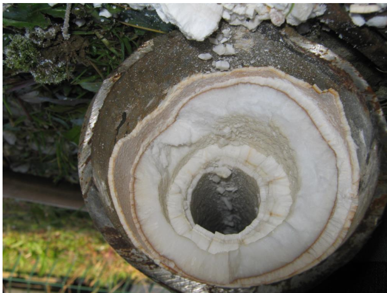
Figure 32: High mineralization and CO 2 degassing of the water cause scaling which clogs the well (Benedikt, Slovenia)
