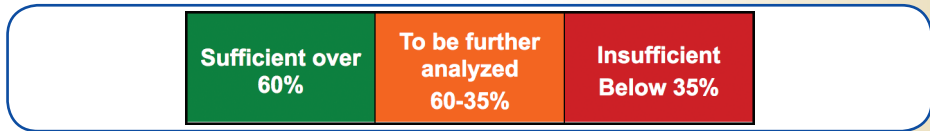
Figure 5: Rule of thumb for first evaluation of actual storage capacity of countries based on withdrawal capacity/peak day consumption ratio
