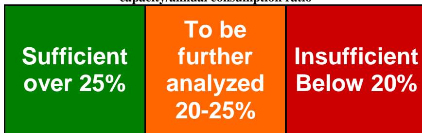
Figure 4: Rule of thumb for first evaluation of actual storage capacity of countries based on working gas capacity/annual consumption ratio
